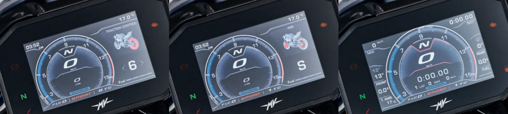
1 TC - TRACTION CONTROL WITH 8 LEVELS + OFF 2 ABS SETTING 3 CHRONOMETER
